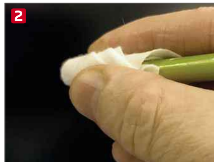
Press the pencil's cloth-covered point on the stuck pixel and massage it gently
